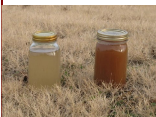
Fig. 1. Simulated run-off from a soil with nearly solid plant residue cover (left) vs. bare soil run-off (right) with a high level of soil erosion. (Photo from NRCS archives.)
